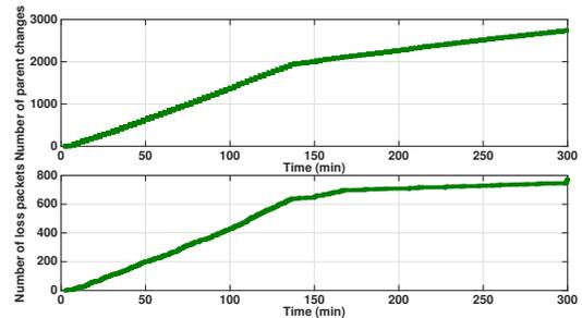
**Figure 2: Number of parent changes and packet loss performance as a function of simulation time.**
