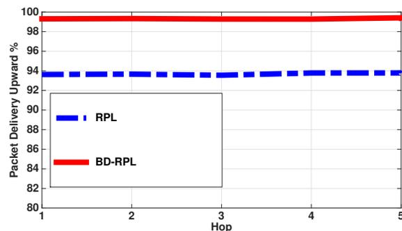
**Figure 7: Upward Packet Delivery Ratio as a function of the hop distance from the sink for RPL and BD-RPL.**
