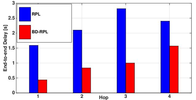
Figure 10: Delay as a function of the hop distance from the sink for RPL and BD-RPL.
