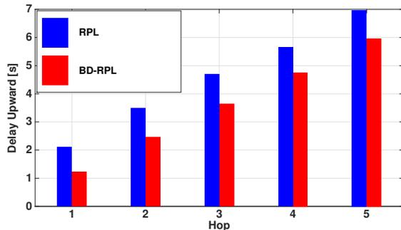
**Figure 5: Upward Average Delay as a function of the hop distance from the sink for RPL and BD-RPL.**
