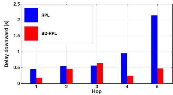
**Figure 6: Average Delay Downward as a function of the hop distance from the sink for RPL and BD-RPL.**
